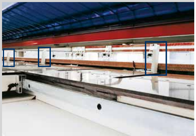
Front alignment devices for the automatic loading.
