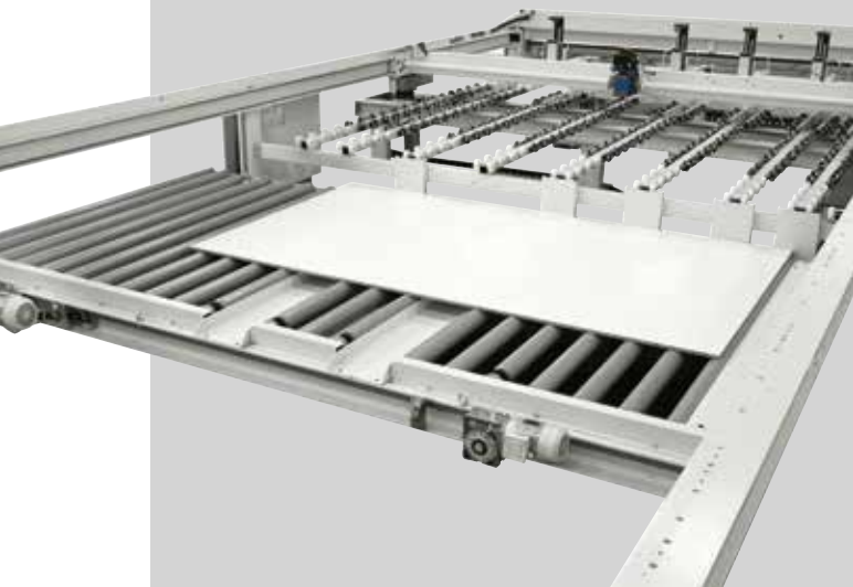
Front alignment devices for the automatic loading.
